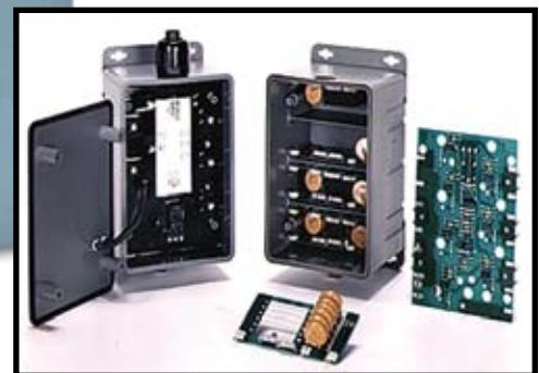
The ASCO PULSAR® 450 provides unparalleled protection from power surges and transients for branch panels or any application where a compact size is necessary. The PULSAR® 450 is a field proven, high performance surge suppressor which limits large surges and transients through a unique array of computer matched, individually fused Metal Oxide Varistors (MOVs).
